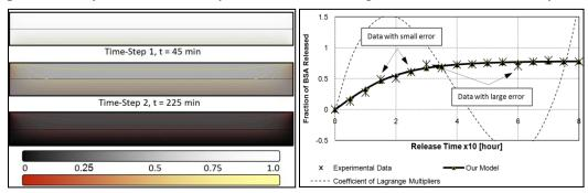
Dynamic of release of BSA from a bi-layer PVA (cycle 1 and 6) obtained from our model (gray-bar) and a validated FE model (color-bar) [2] (right) – fraction of BSA released, and experimental and modeling data of the BSA release from the cycle 6-PVA (left). **Conclusion**
