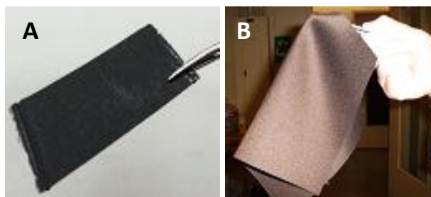
Fig. 1: Stiff PPy/PLLA membrane (A) and flexible PPy-coated PET fabric (B).
