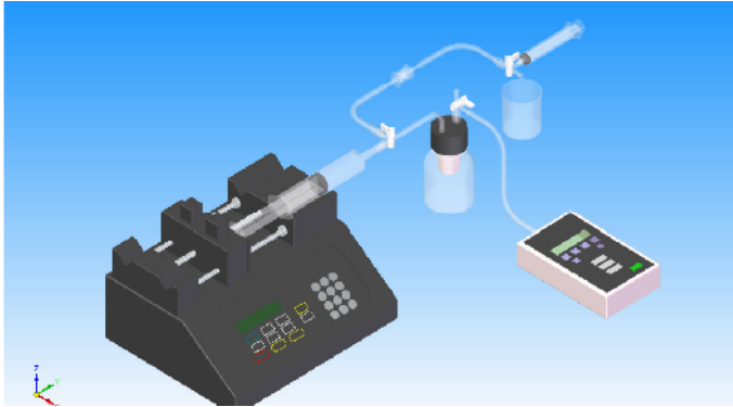
Fig 1. Schematic representation of the bench test used to characterize gel occlusive properties
